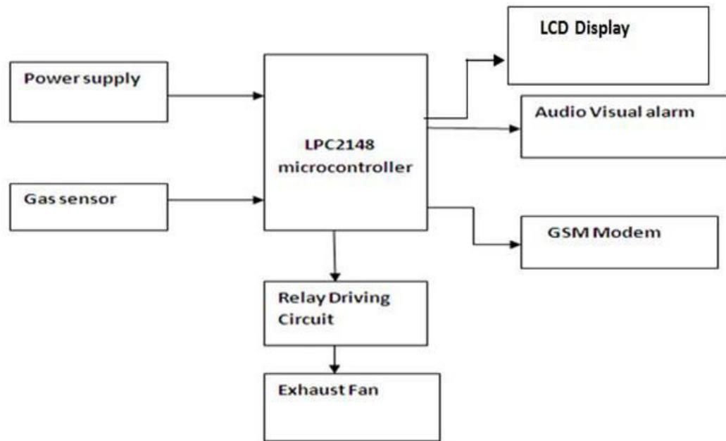
Figure 3: The System Block Diagram
