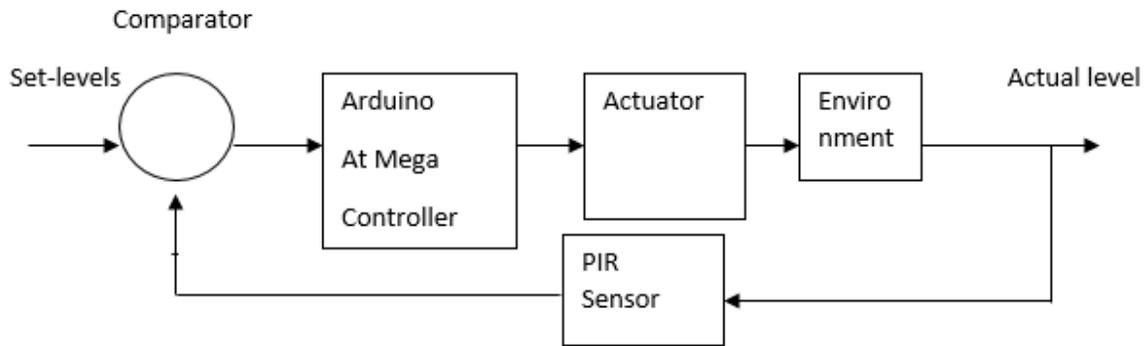
Figure 1: Block Diagram of Proposed Intruder Detection Security System
